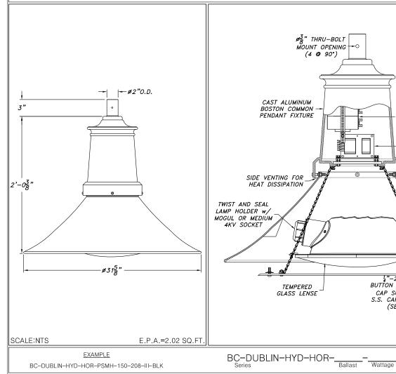
CAPACITOR & STARTER QUICK DISCONNECT HID BALLAST SAFETY CHAIN w/ HEAT SHRUNK LATEX SLEEVE SEALED OPTIC CHAMBER HYD-HOR REFLECTOR TYPE III DISTRIBUTION 1"-20x1" S.S. BUTTON HEAD SOCKET CAP SCREW w/ 1/3" S.S. CAPTIVE WASHER (SET OF 4)
