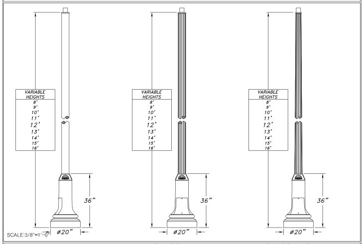
SX-20-S5-\_\_\_ 5" dia. smooth shaft 8'-16' in height SX-20-F5-\_\_\_ 5" dia. fluted shaft 8'-16' in height SX-20-TF35-\_\_\_ 3"-5" dia. tapered fluted shaft 8'-16' in height
