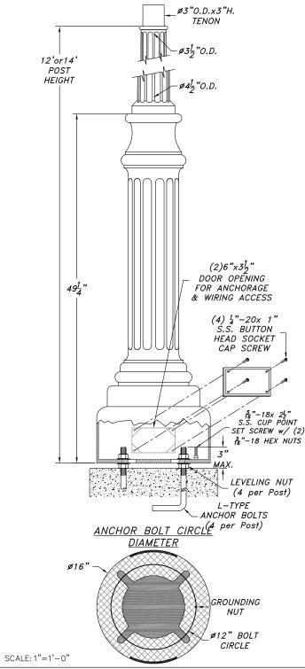
Cast Shrewsbury Series-16" Base-Cast \_\_\_\_ Tapered
