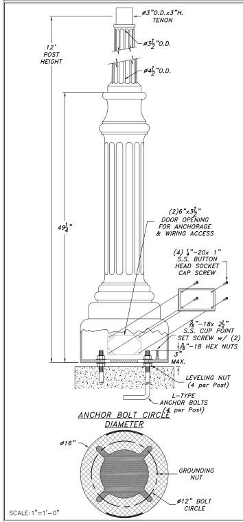
Cast Shrewsbury Series-16" Base-Cast Iron Tapered
