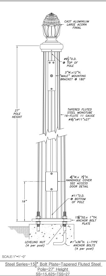
WIRING ACCESS DOOR DETAIL **4¾"**W.x7¾"H. HANDHOLE COVER 1/2"-20x 1" S.S. HEX HEAD CAP SCREW w/ 1" S.S. FLAT WASHER (SET OF 2) (P) 0 0 4¼"W.x7¼"H. OPENING FOR WIRING ACCESS w/ (2) ½"-13 HEX NUTS (@ 0°) (2) ½"-13 GROUNDING HEX NUT 1.7-13x 1.7 S.S. SOCKET HEAD CAP SCREW SCALE:NTS
