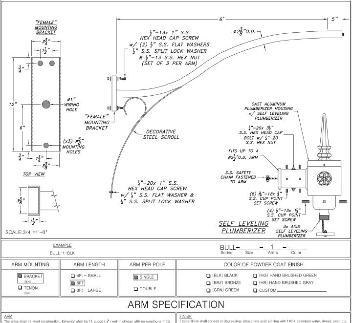
The arms shall be steel construction. Extrusion shall be 11 guage ( $\frac{1}{3}$ ) wall thickness with no warping or mold shifting. Electrical wiring shall run through arm up and out throught the  $\otimes 3$ ° opening.
